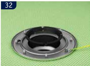
**(UK)** To establish weep holes and to center the upper part over the lower part, cut 1 – 4 notches out of the sealing ring (marked).
