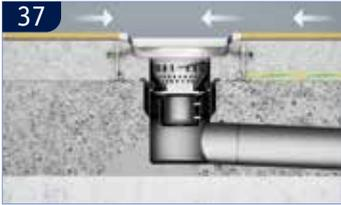
**(UK)** Sectional view showing the completed installation.
