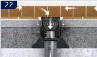
**(UK)** Sectional view showing the completed installation.
